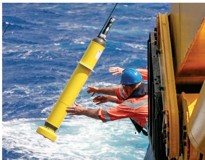
Scientists deploy an Argo float. For over a decade, more than 3000 floats have provided near-global data coverage for the upper 2000 m of the ocean.
