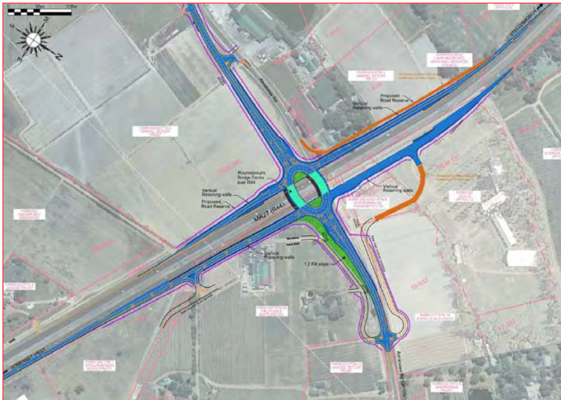
Figure 6-7: R44/Annandale Road grade-separated roundabout with vertical retaining walls
