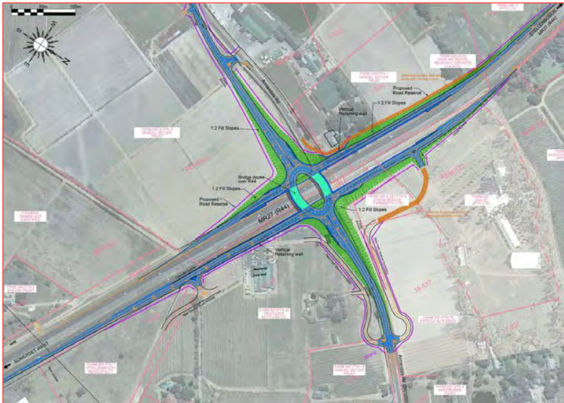
Figure 6-6: R44/Annandale Road grade-separated roundabout with ramp embankments
