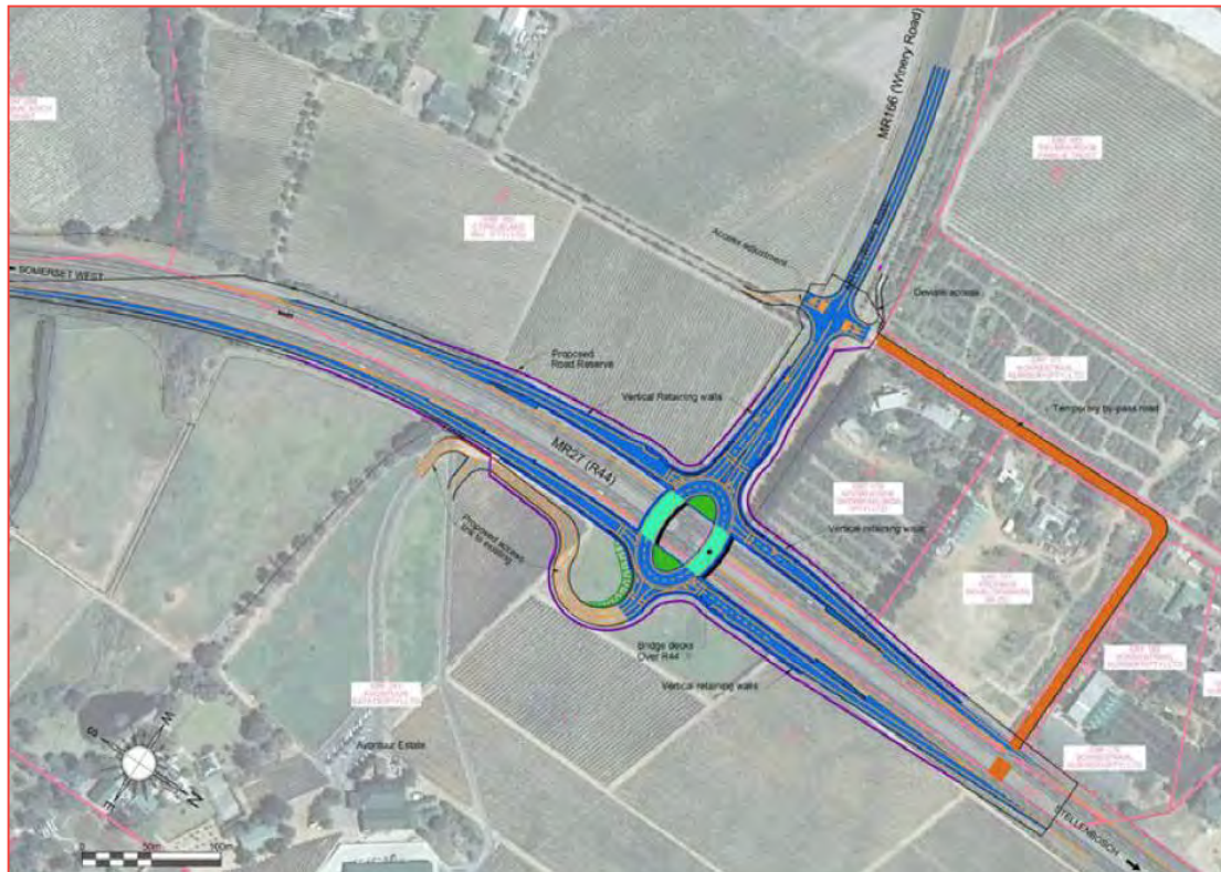
Figure 6-4: R44/Winery Road grade-separated roundabout with vertical retaining walls
