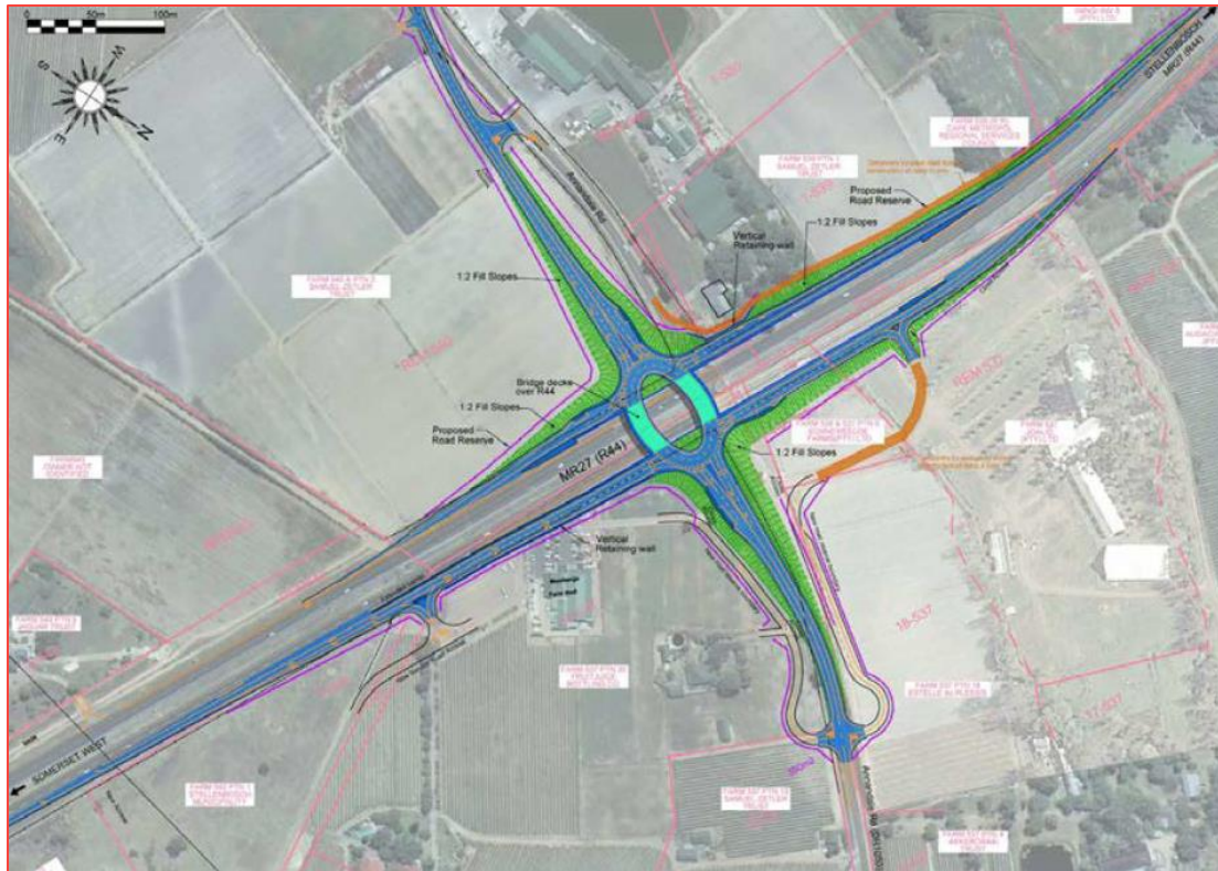
Figure 6-6: R44/Annandale Road grade-separated roundabout with ramp embankments Source: Kantey & TEMPLER
