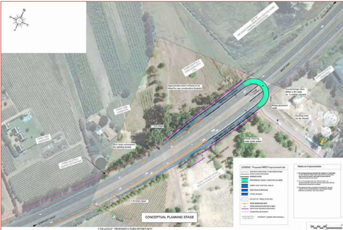
Figure 6-9: R44/Jamestown grade-separated U-turn facility
