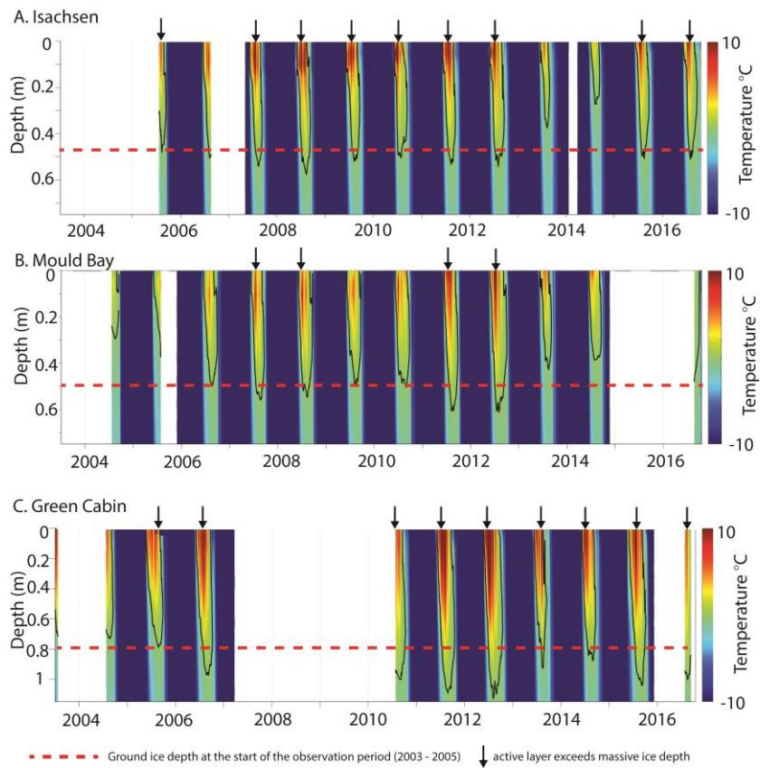
**Figure 3.** Thaw depth and temperature diagrams for: A. Isachsen, B. Mould Bay, and C. Green Cabin. Red dotted line shows ground ice depth at the start of the observation period. Black arrows indicate years where maximum thaw depth exceeds ground ice depth. The black continuous line is the 0°C isotherm in the ground.
